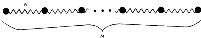
Figure 3. A linear sequence of hierarchical models which yields a system that is described by a one-dimensional convective-diffusion equation.
